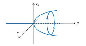
The origin loses stability at  $\mu = 0$  and a stable limit cycle emerges.
