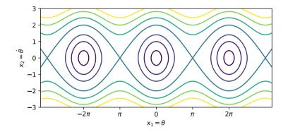
Phase portrait of the pendulum for the undamped case k = 0.
