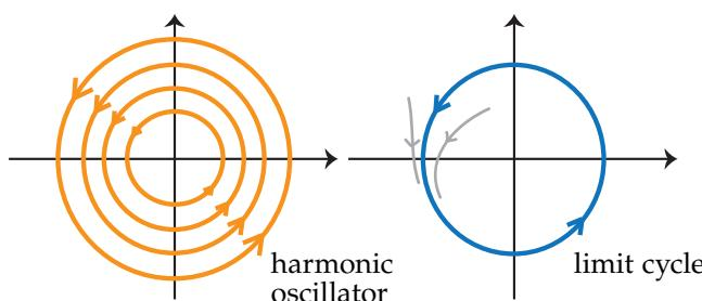
Example: van der Pol oscillator (models a system with self-sustained oscillations)
