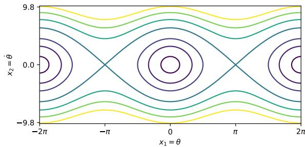
Figure 1: Phase portrait of the pendulum for the undamped case  $k = 0$  with  $m = 1$ ,  $g = 9.8$ ,  $\ell = 1$ .
