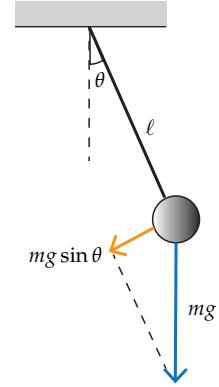
The damping torque acting on the pendulum is  $-\ell(k\ell\theta)$  for the planar pendulum.
