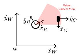
The mobile robot obtains measurements of it's orientation using an inertial measurement unit (IMU) that provides us with angular velocities. We can then compute the exponential map at each time step to obtain how the orientation of the robot changes over time. For example, if the angular velocity readings of the robot are  $\omega(t) = [0, 0, 0.1]^{T}$ :
