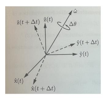
If we examine the body frame at times t and  $t+\delta t$ , the change in frame orientation can be described as a rotation of angle  $\delta\theta$  about some unit axis  $\hat{\omega}$  passing through the origin. As the limit  $\delta t\to 0$ , we can define the angular velocity  $\omega$  as:
