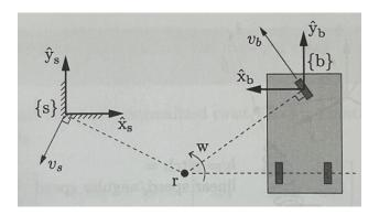
This example shows the top view of a car, with a single steerable front wheel driving on a plane. The angular velocity caused the rotation of the front wheel is  $\mathbf{w} = 2$  rad/s about point r. We can write the point of rotation in reference to either s or b as:
