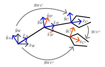
where  $g_{WC}$  represents the first configuration we solved for in reference to the world frame W, and  $g_{WC'}$  represents the second configuration, again in reference to the world frame W.
