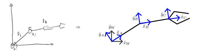
We can solve for the end-effector configuration  $g_{WC}$  using the homogeneous coordinates:
