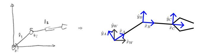
where we solved for the end-effector configuration  $g_{WC}$  (the transformation of frame C with respect to the world frame) as:
